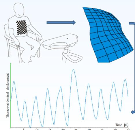
Figure 1. Working principle of SLP.
